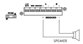
SPEAKERS NEGATIVE TERMINALS ON AMPLIFIER ARE NOT USED IN BRIDGED MODE BRIDGING IS DONE BY SUMMING POSITIVES.
